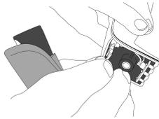
7. Connect the battery cable connector to the handle board.
