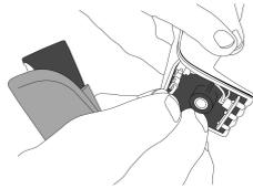
3. Disconnect the battery cable connector from the handle board.
