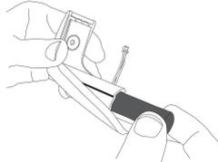
4. Remove the used battery from the battery container.
