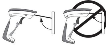
2. The scan line must cross the entire barcode. The imager can not read the barcode data without seeing the entire barcode.
