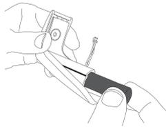
6. Place the new battery into the battery container.
