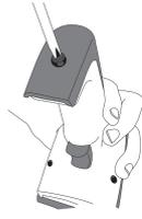
1. Loosen the screw at the bottom of the imager.
