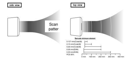
Scanning a bar code label with a presentation scanner is very simple: present the product's bar code label to the scanner as illustrated in the figure below.
